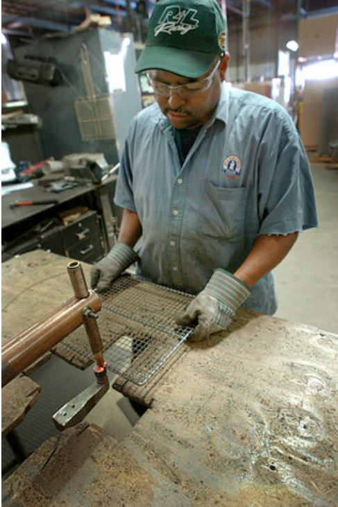
Hector Carmona welds a basket prototype at Marlin Steel that will then be mass-produced by robotic fabricating equipment. (Sun photo by Glenn Fawcett / September 5, 2007)
