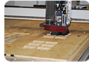
The CNC machine uses recycled sawdust to create go/no-go fixtures for quality inspections. Source: Marlin Steel Wire Products LLC
