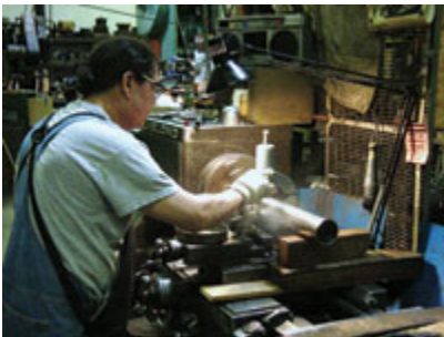
Quality Float Works employee Ramiro Bocanegra performs a trimming process using a lathe.
