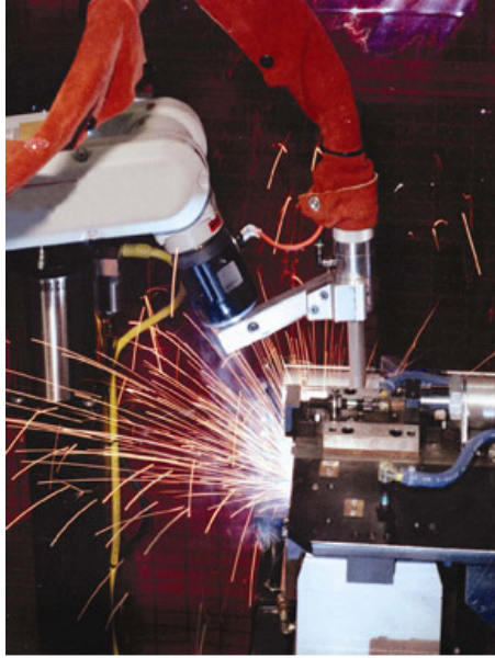
Shown is the heavily fixtured robotic welding of a basket for Toyota. A finished cleaning basket used by Boeing to wash parts.
